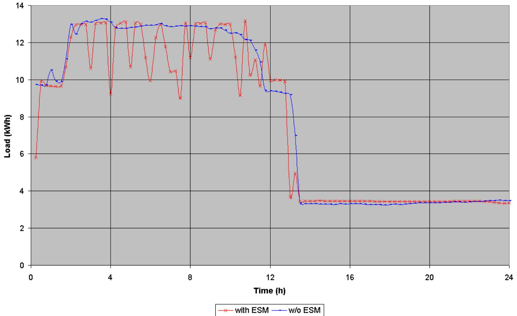
Figure 2. 15-minute average ID room load (kWh) vs time (2<sup>nd</sup> ESM on test and baseline).
