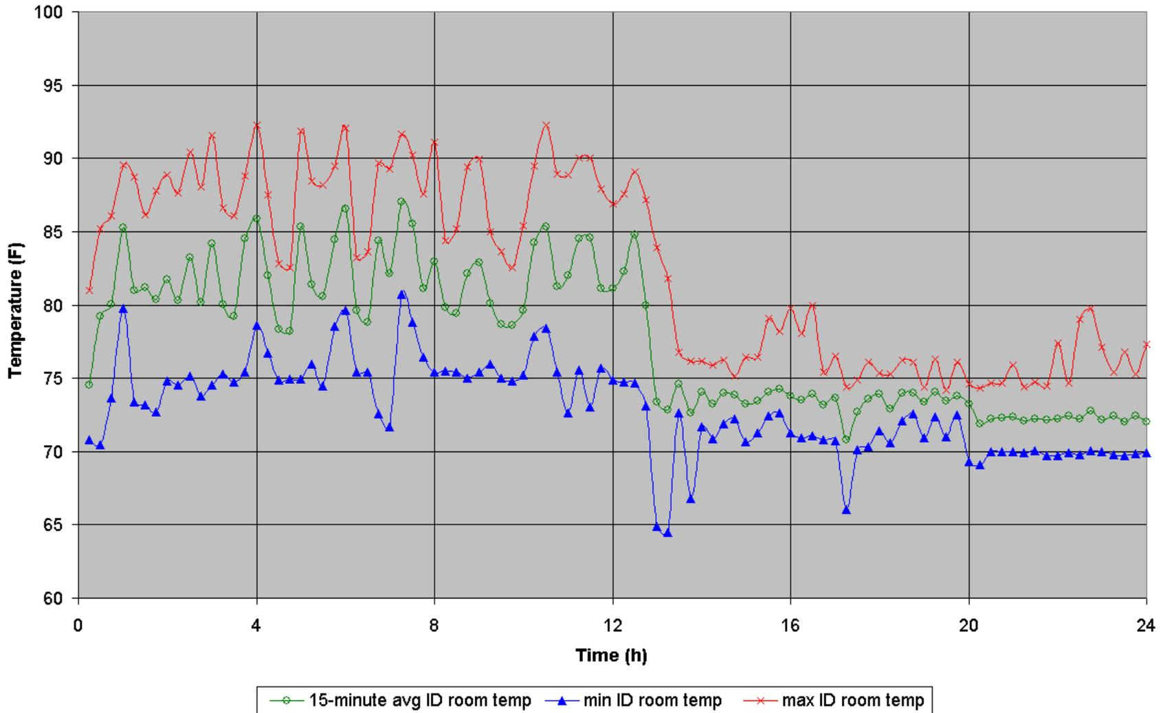
Figure 4. Average, minimum and maximum ID room temperatures for 2<sup>nd</sup> ESM on test.
