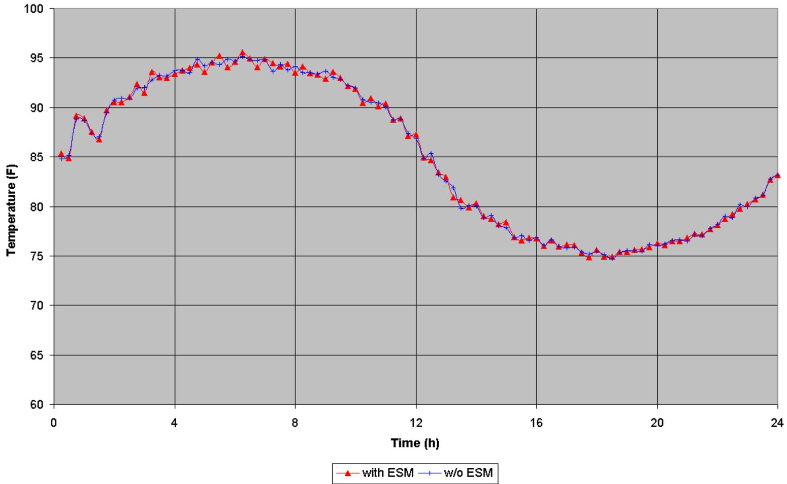
Figure 1. 15-minute average OD room temperature vs time (2<sup>nd</sup> ESM on test and baseline).
