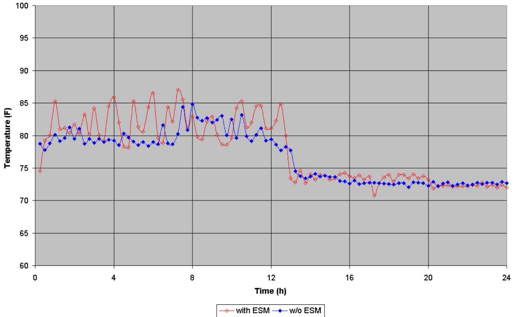
Figure 5. 15-minute average ID room temperatures vs time (2<sup>nd</sup> ESM on test and baseline).
